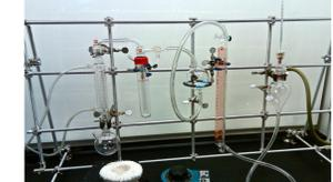
Figure 7. Apparatus used for hydrolysis of NaBH<sub>4</sub>
