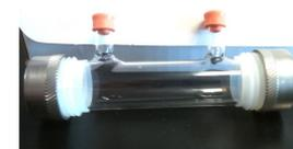
Figure 7. Gas Tube for IR
