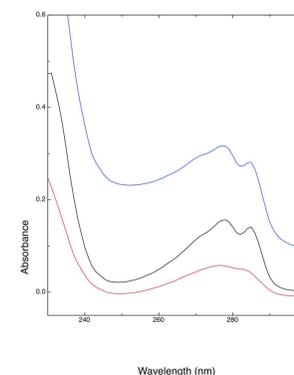
UV/Visible spectra of BPA: 5 ppm in CH<sub>2</sub>Cl<sub>2</sub> (black line), in CH<sub>2</sub>Cl<sub>2</sub> after liquid/liquid transfer from 5 ppm in H<sub>2</sub>O (blue line), and 5 ppm in H<sub>2</sub>O (red line). Note that 5 ppm in H<sub>2</sub>O corresponds to a molar concentration about 1.33 x that corresponding to 5 ppm in CH<sub>2</sub>Cl<sub>2</sub>.
