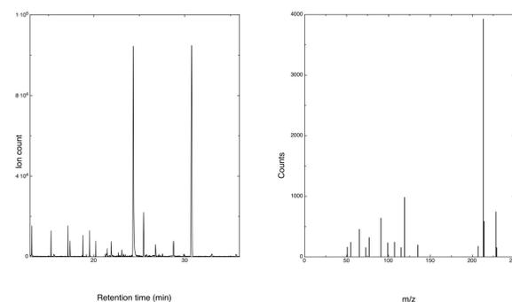
Chromatogram from SPME BPA sample (67 ppm). The BPA peak occurs near 24 minutes. The small peak at 25 minutes is due to BPA diacetyl derivative. The peak at 31 minutes diisooctyl phthalate from the vial septum.
